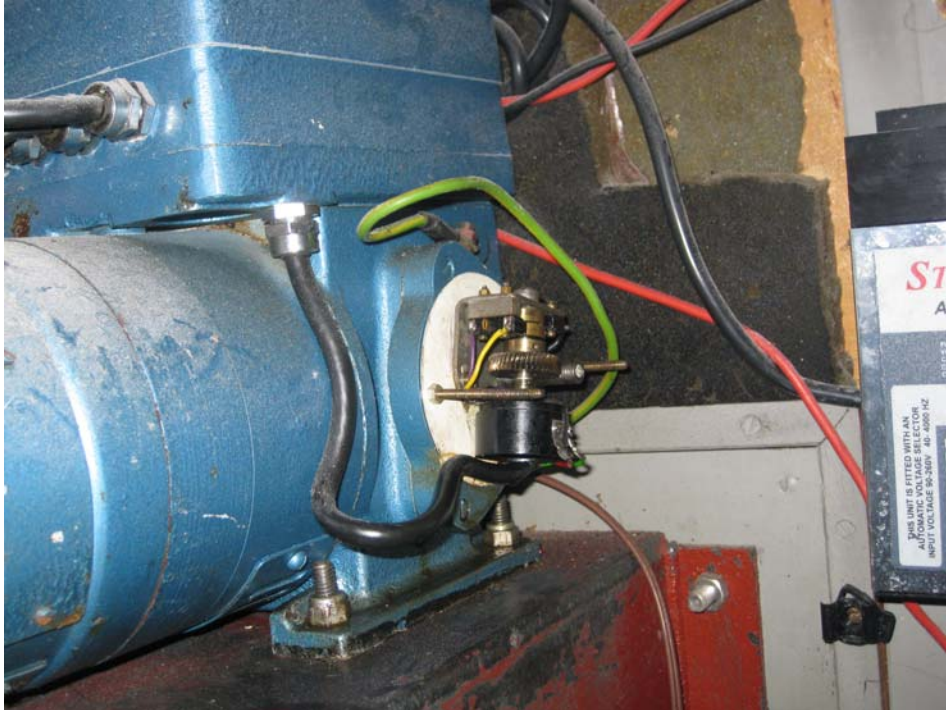
Figure 7. Position of the rudder feedback assembly on the side of the Drive Unit. The black 7-core cable from the feedback assembly to the Relay Box is clearly visible (photograph by N.Kassel) .
