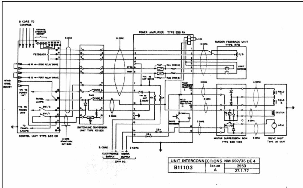
**Figure 1.** Original block scheme (extracted from the Neco Manual) of the circuitry that controls the Neco Type 35DE4 Drive. The Clutch is always activated during Auto Mode while the Armature and one Field is activated whenever the motor is required to turn. The Armature is powered with fixed polarity while the motor turning direction depends on which of the two Fields is activated.
