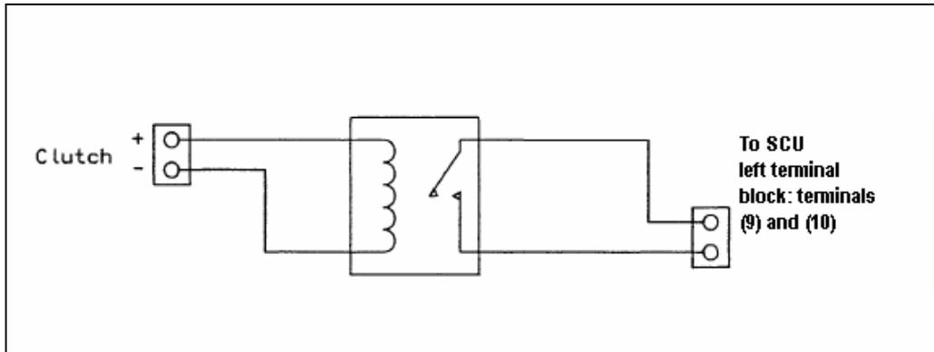
Figure 5. Relay interface for the Clutch.
