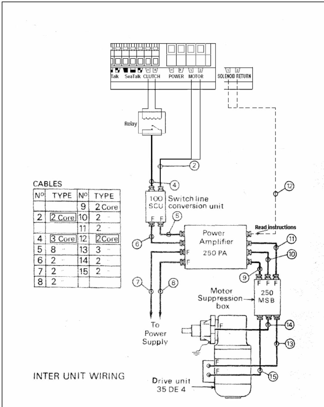
**Figure 7.** Inter Unit wiring after modification. The cables that need modification are boxed in the table. Cable N.4 is marked as 3-core because it is so in the original setup; actually only 2 cores are needed.
