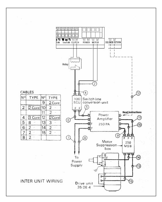
**Figure 7.** Inter Unit wiring after modification. The cables that need modification are boxed in the table. Cable N.4 is marked as 3-core because it is so in the original setup; actually only 2 cores are needed.
