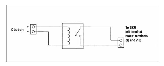
Figure 5. Relay interface for the Clutch.
