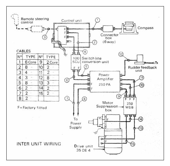
**Figure 6**. Original Neco Inter Unit wiring before modification (extracted from the Neco Manual).
