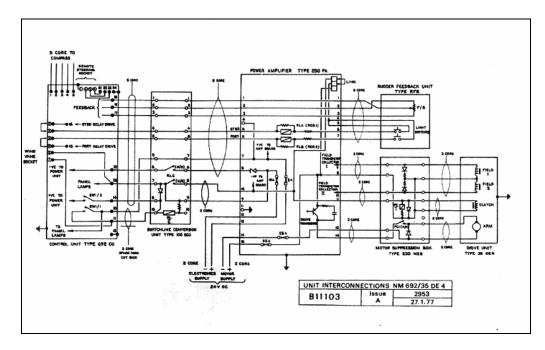
**Figure 1.** Original block scheme (extracted from the Neco Manual) of the circuitry that controls the Neco Type 35DE4 Drive. The Clutch is always activated during Auto Mode while the Armature and one Field is activated whenever the motor is required to turn. The Armature is powered with fixed polarity while the motor turning direction depends on which of the two Fields is activated.
